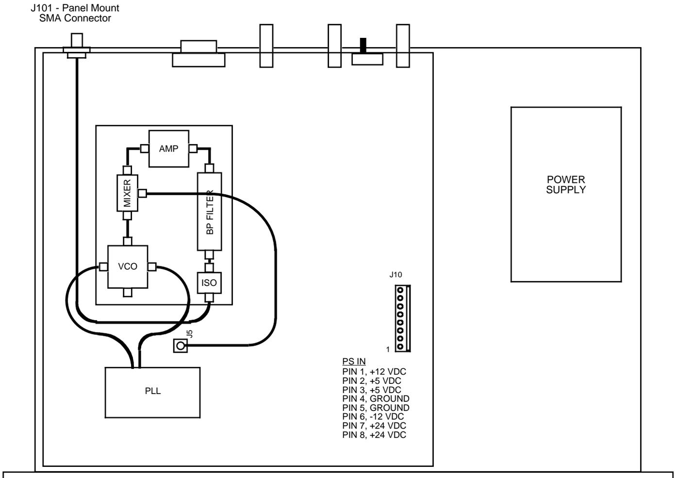
FIGURE 2.0 2115-109# Mechanical Assembly
